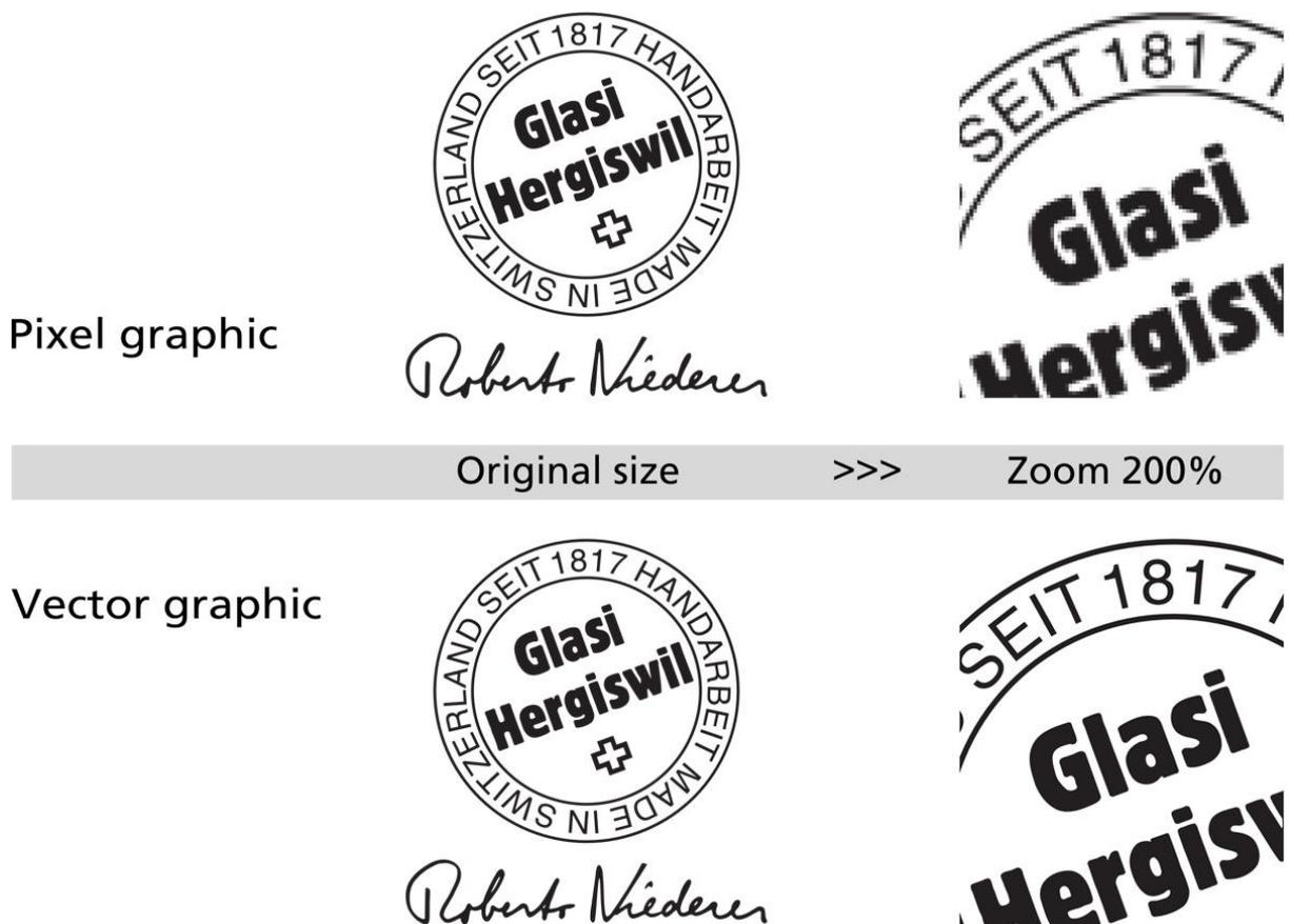
A pixel graphic is made up of individual pixels, and is usually unsuitable for use. Scaling causes a reduction of quality in pixel graphics. Almost all computer and Internet graphics are pixel graphics.
