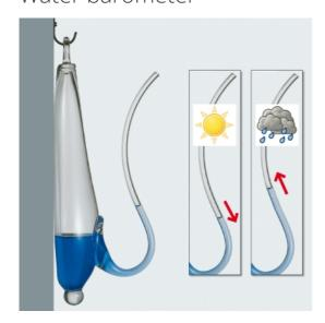
The water barometer, or "Goethe glass", shows the air pressure and therefore the coming weather. Fill the barometer as shown with distilled water, which can also be dyed, and hang it somewhere indoors. If the water climbs up the spout, the weather is bad, if it comes back down again, it will be fine. Note: If the water overflows you need to add some more water straight away. Very few glass blowers have mastered the art of blowing this object to perfection.
